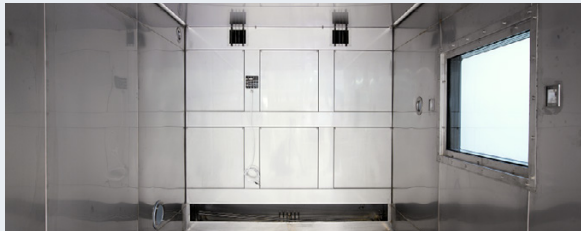
WALK-IN TEST CHAMBERS
